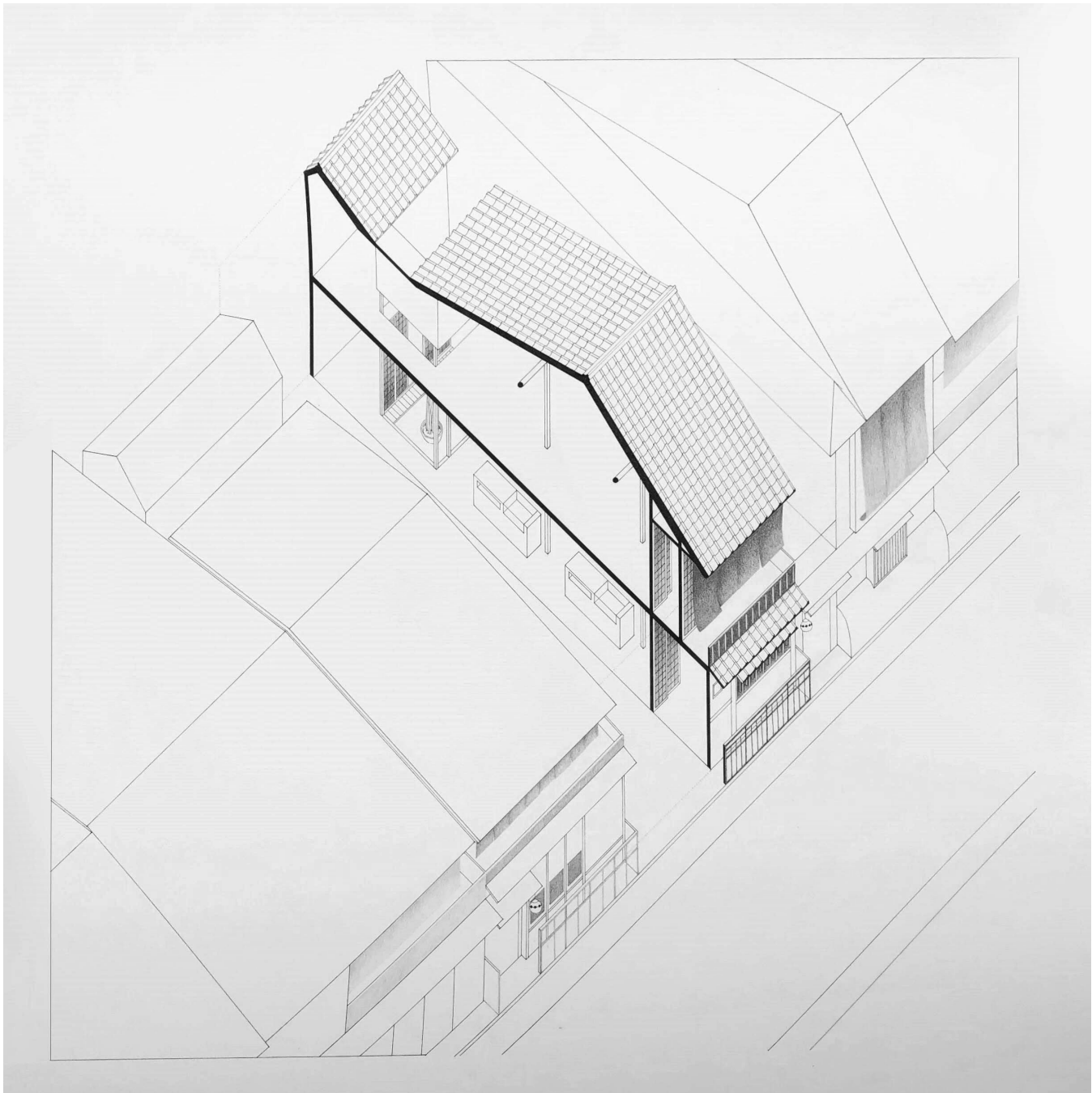
Figure 8. Cutaway axon Leica store in a renovated machiya (rowhouse) in Gion District of Kyoto. Drawing by Virginia Tech architecture student Jessica Wirth (2019).
